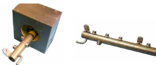
Fig. 2: Coil with test piece
